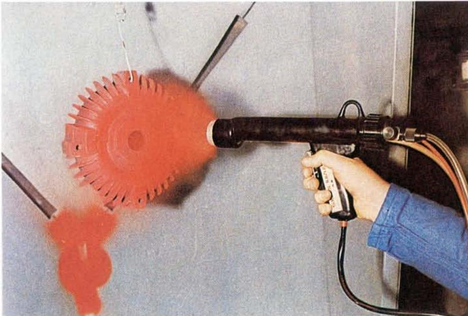
Two of our chemicals companies have pioneered electrostatic powder-coating which has a wide variety of industrial applications. Here the cover for an electric motor is being coated with an epoxy resin-based powder.
